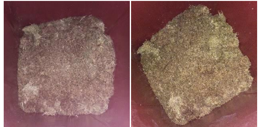
Food waste after mincing and dewatering processes
